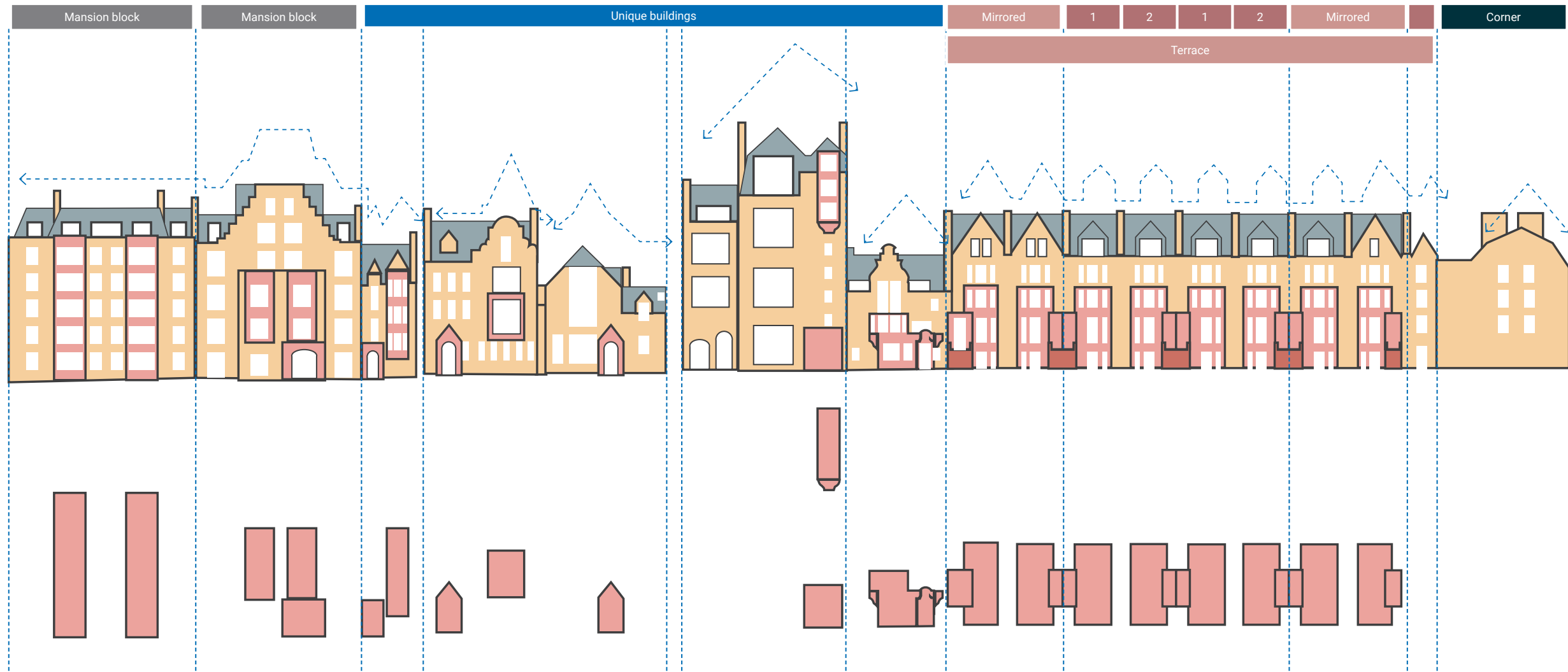
Diagrammatic study of the rhythm, roof variation, window variety and bay positions on 26-58 Tite Street.
